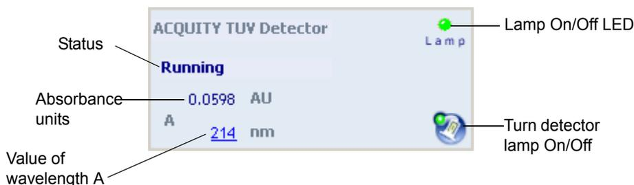
The TUV detector control panel displays absorbance units and wavelength values. You can edit these parameters when the system is idle by clicking on the underlined value. You cannot edit detector parameters while the system is running samples.
