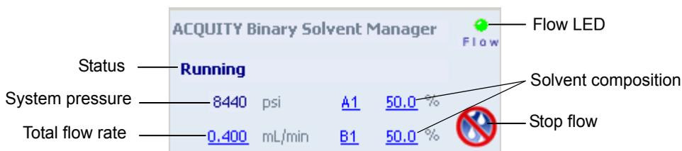
The binary solvent manager control panel displays flow status, system pressure, total flow rate, and solvent composition parameters.
